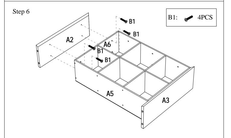
Assemble Left Side Panel A2 to Side Panel A6 using Bolts B1 as shown above.
