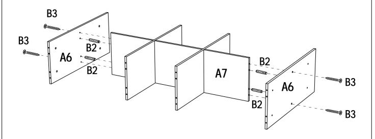
Assemble Side Panels 6 to Cross Panel A7 using Wood Dowels B2 &Screws B3 as shown above. Page 5 of 8  $\,$
