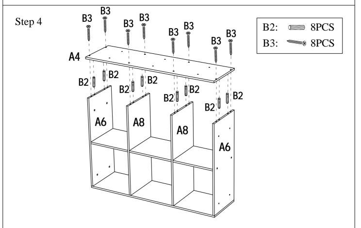
Assemble Small Top Panel A4 to Side Panels 6 & Center Dividers A8 using Wood Dowels B2 &Screws B3 as shown above.
