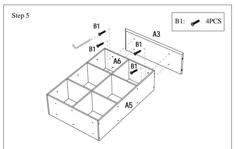
Assemble Right Side Panel A3 to Side Panel A6 using Bolts B1 as shown above.
