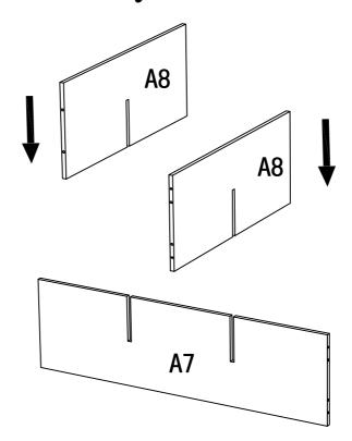
Insert Center Dividers A8 into Cross Panel A7 as shown above.
