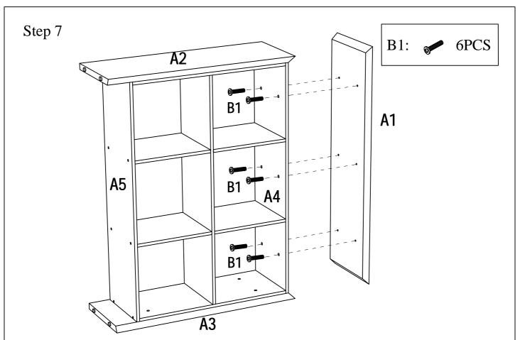
Assemble Top Panel A1 to Small Top Panel A4 using Bolts B1 as shown above.
