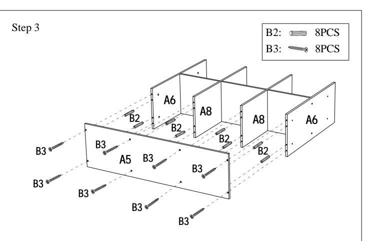
Assemble Side Panels 6 & Center Dividers A8 to Bottom Panel A5 using Wood Dowels B2 &Screws B3 as shown above.
