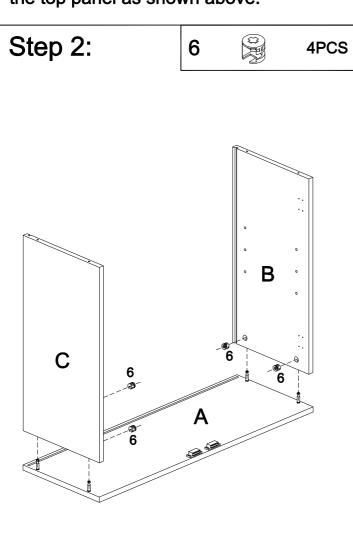
Assemble Side Panels(C&B)to Top Panel (A) using Cam-locks&bolts(5&6) as shown above.
