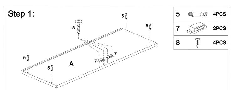
Assemble Magnets(7) to Top Panel(A) using screws(8), then tighten Cam-bolts(5) to the top panel as shown above.
