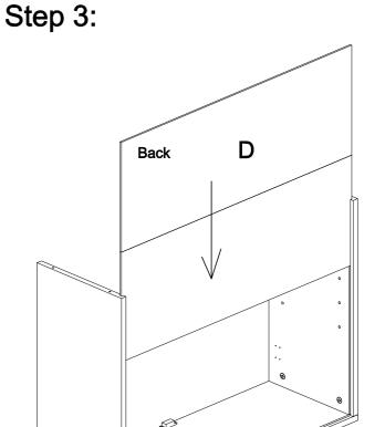
Insert Back Panel (D) into the grooves on Side Panels as shown above.
