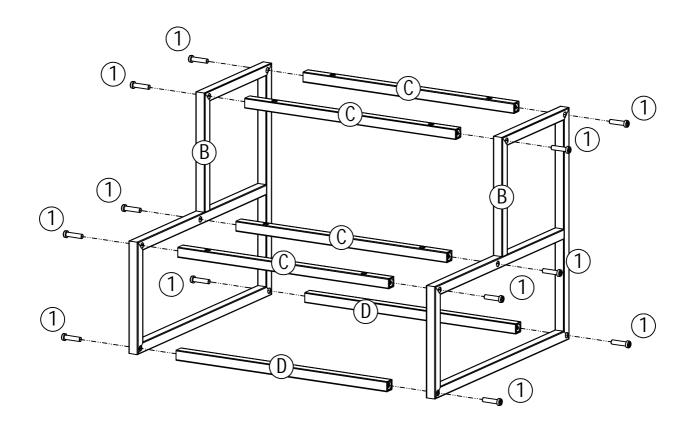
Assemble Connecting Bars(C) &(D) to Side Frames(B) using Bolts (1) as shown above.
