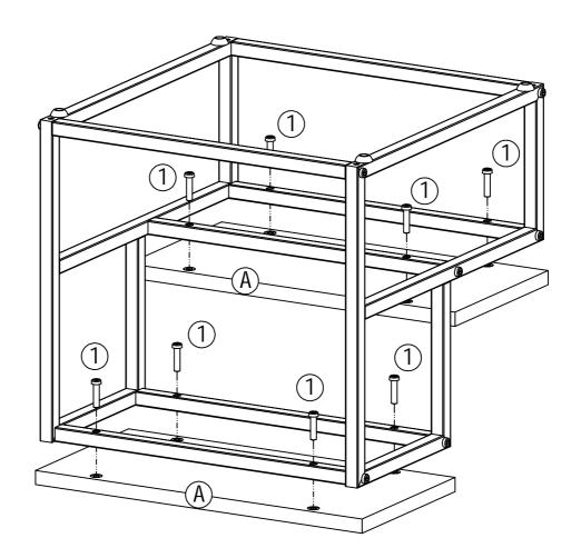
Assemble Top Panels(A) to Connecting Bars(C) using Bolts(1) as shown above.
