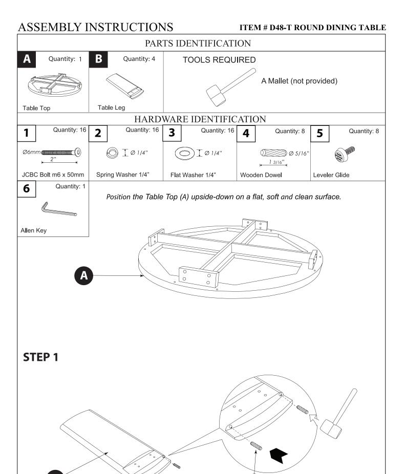
Insert the wooden dowels (4) into the designated holes in all table legs (B) until the dowels fit snugly in each hole.
