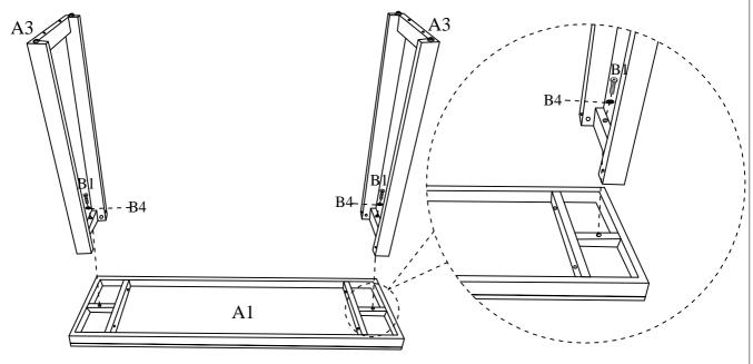
Do not fully tighten Bolts until Step 2.
