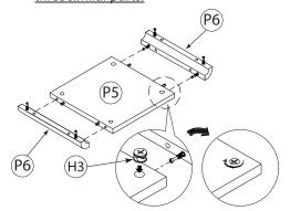
Align the Camlock (H3) & use a screwdriver to turn it to locked position when it is connected to the bolt.
