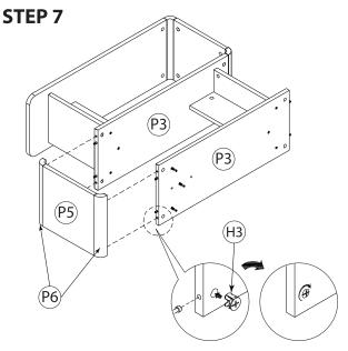
Align the Camlock (H3) & use a screwdriver to turn it to locked position when it is connected to the bolt.
