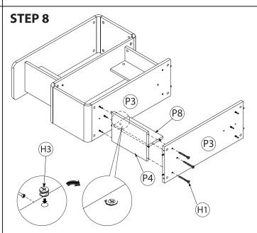
Align the Camlock (H3) & use a screwdriver to turn it to locked position when it is connected to the bolt.
