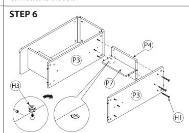
Align the Camlock (H3) & use a screwdriver to turn it to locked position when it is connected to the bolt.
