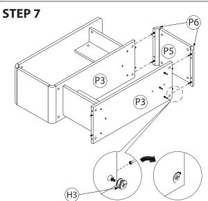
Align the Camlock (H3) & use a screwdriver to turn it to locked position when it is connected to the bolt.
