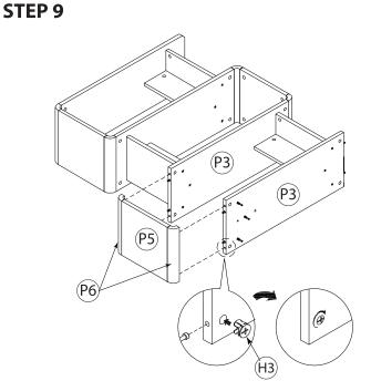
Align the Camlock (H3) & use a screwdriver to turn it to locked position when it is connected to the bolt.
