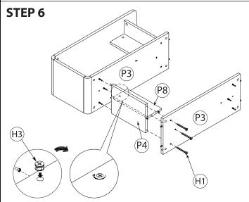
Align the Camlock (H3) & use a screwdriver to turn it to locked position when it is connected to the bolt.
