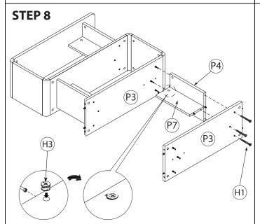
Align the Camlock (H3) & use a screwdriver to turn it to locked position when it is connected to the bolt.
