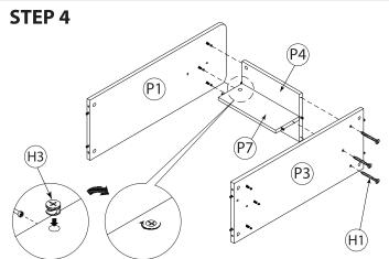
Align the Camlock (H3) & use a screwdriver to turn it to locked position when it is connected to the bolt.
