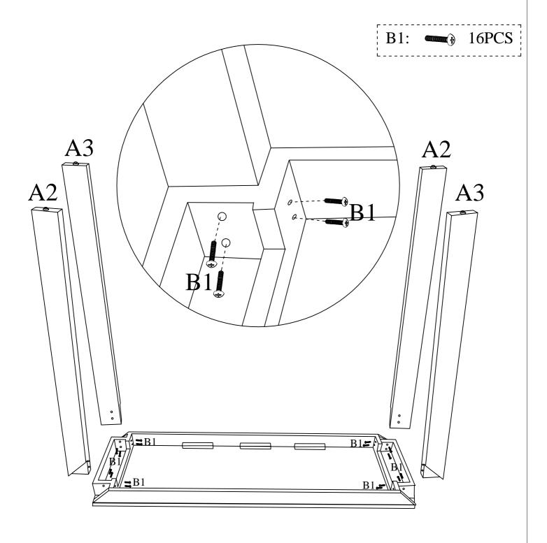
Assemble Legs A2 &A3 to the bottom of Table top A1 using Bolts B1 as shown above.
