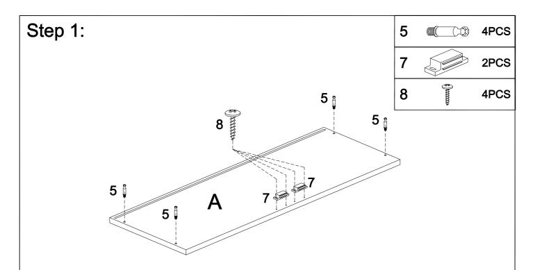
Assemble Magnets(7) to Top Panel(A) using screws(8), then tighten Cam-bolts(5) to the top panel as shown above.
