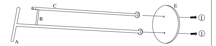
Assemble Front Pole (A) & Rear Pole (C) to Base (E) using Bolts (1) as shown above. Please tighten all bolts at this point.
