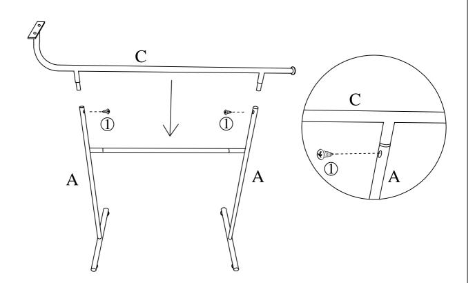
Insert Connect Bar (C) into Legs(A) using Screws (1) as shown above.
