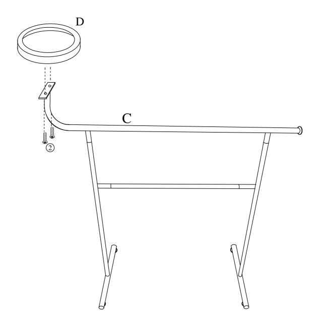
Assemble Top Tray (D) to Connecting Bar (C) using Bolts (2) as shown above.
