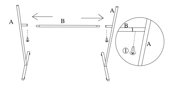
Insert Connect Bar (B) into Legs(A) using Screws (1) as shown above.
