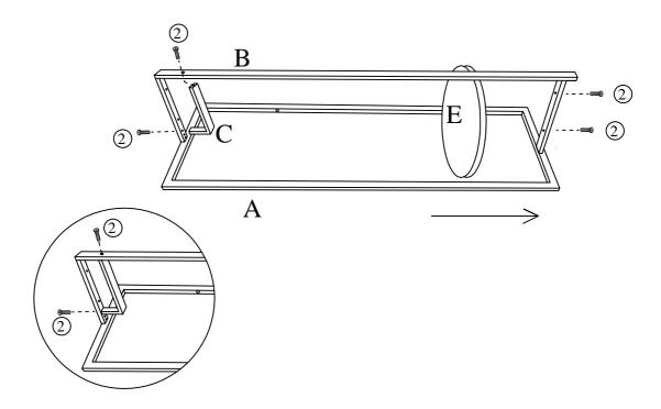
Assemble Coat Hook (C) to Rear Frame (B) using Bolts (2) as shown above. Then attach Bottom Panel (E) to Rear Frame (B) using Bolts (2).
