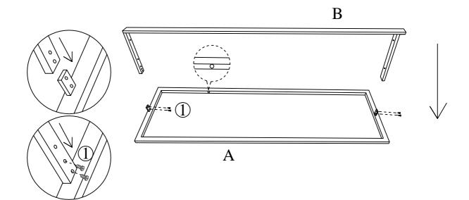
Assemble Rear Frame (B) to Front Frame (A) using Bolts (1)as shown above. Please do not tighten bolts until the last step.
