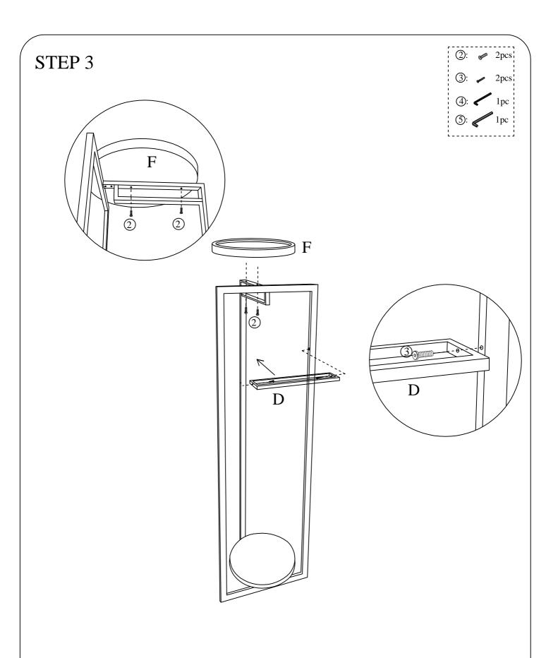
Assemble Hook (D) to Front Frame (A) using Bolts (3) as shown above. Then attach Top Tray (F) to Rear Frame (B) using Bolts (2). Please tighten all bolts at this point.
