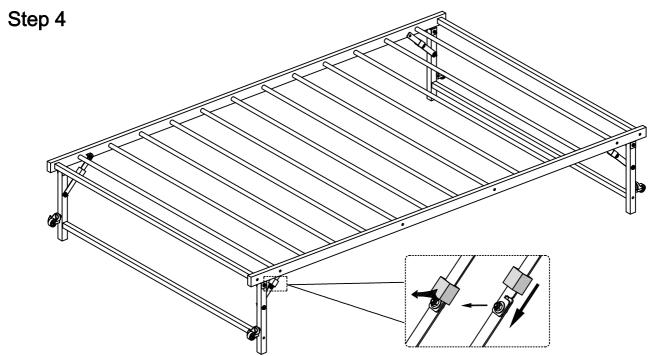
After the caps are slid into place, double- check to make sure they are securely fitted. If necessary, adjust them until they are flush with the surface and provide full coverage.
