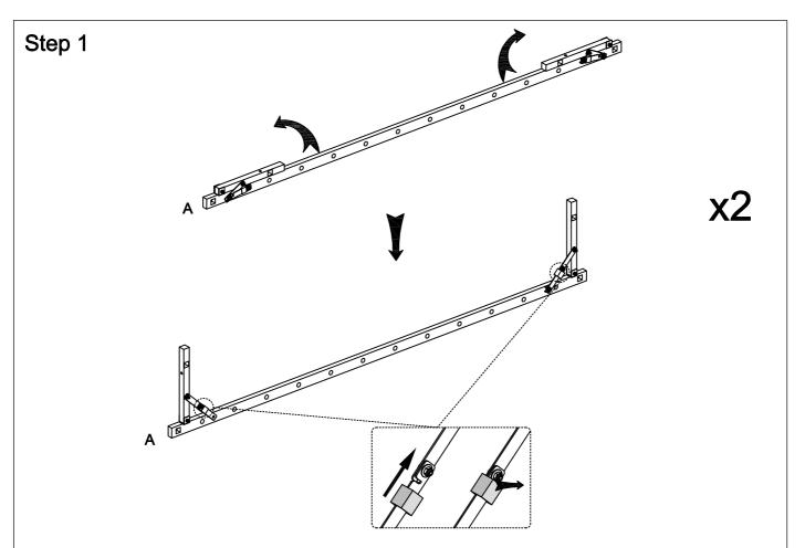
Unfold the legs and slide the protective metal caps over the connecting point as shown above.
