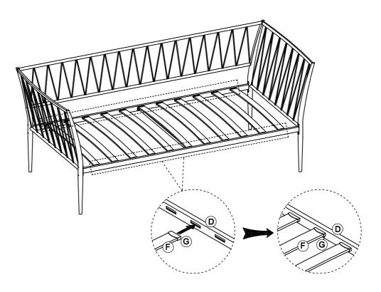
Insert Plastic Caps (G) into holes on Side Rails (D) as shown above. Please tighten all bolts at this point.
