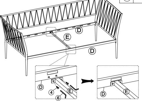
Assemble Support Bar (E) to Side Rails(D) using Bolts (4) as shown above, do not tighten bolts until Step 5.
