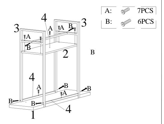
Assemble Connect Bars (4) to Side Frames (3) using Bolts (B) as shown above, then assemble shelf to Side Frames(3)using Bolts(A) as shown above.
