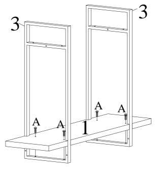
Assemble Top Panel (1) to Side Frames (3) using Bolts (A) as shown above.
