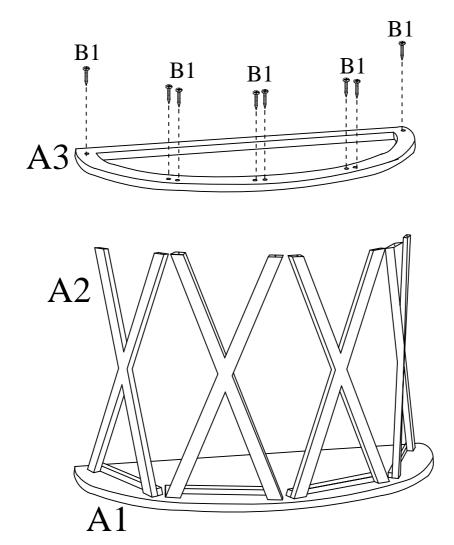
Assemble Bottom Frame A3 to Support Frames A2 using Screws B1 as shown above.
