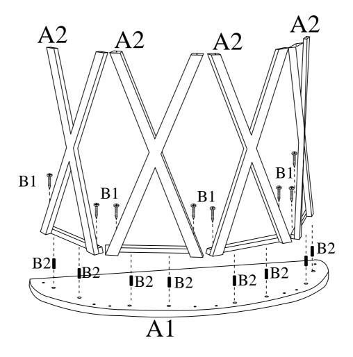
Assemble Support Frames A2 to the bottom of Top Panel A1 using Screws B1 & Wood Dowel B2 as shown above.
