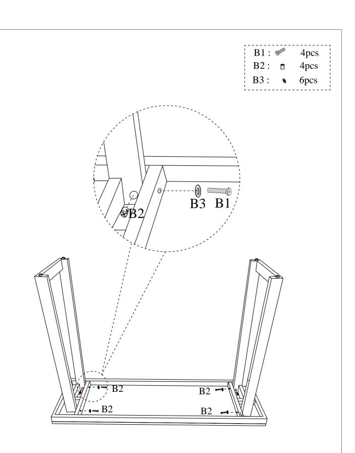
Do not fully tighten Bolts until all of the bolts are attached.
