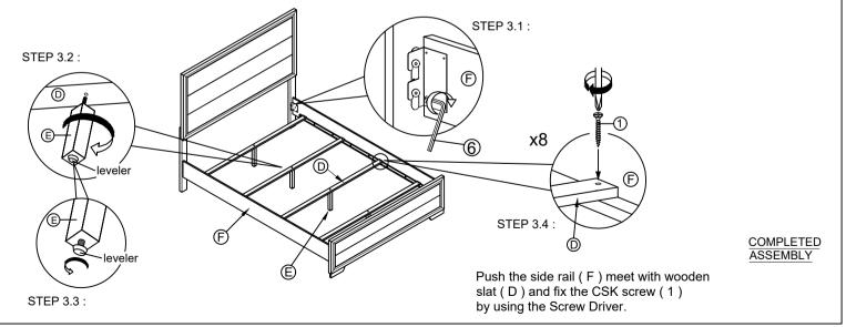
NOTE: MUST TIGHTEN SCREWS PERIODCALLY WITH USE SCREW WILL BECOME LOOSE CHECK TIGHTNESS OF ALL SCREW EVERY 6-8 WEEKS.
