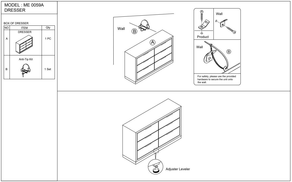
NOTE : MUST TIGHTEN SCREWS PERIODCALLY WITH USE SCREW WILL BECOME LOOSE CHECK TIGHTNESS OF ALL SCREW EVERY 6-8 WEEKS.
