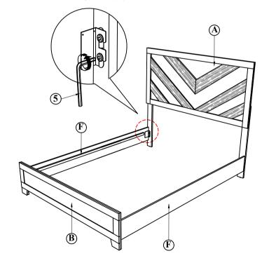
STEP 3: Tighten the 4 Corner with Allen Key (5). Fix the Bed Slat Support Leg (E), to Bed Slat (D) as shown. Install the bed slat (D) to side rail (F) and tighten with Csk Screw (6) as per diagram shown. (NOTE: THE SETUP MUST DONE AT THE DECIDED LOCATION FOR THE BED TO OBTAIN PERFECT STABILITY)
