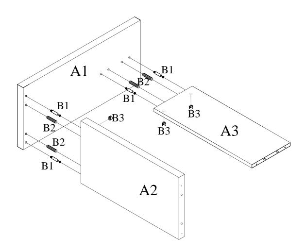
Assemble Side Panel A2 & Divider A3 to the bottom of Top Panel A1 using Cam-Bolts B1 & Cam-Nuts B3, and Wood Dowels B2 as shown above.
