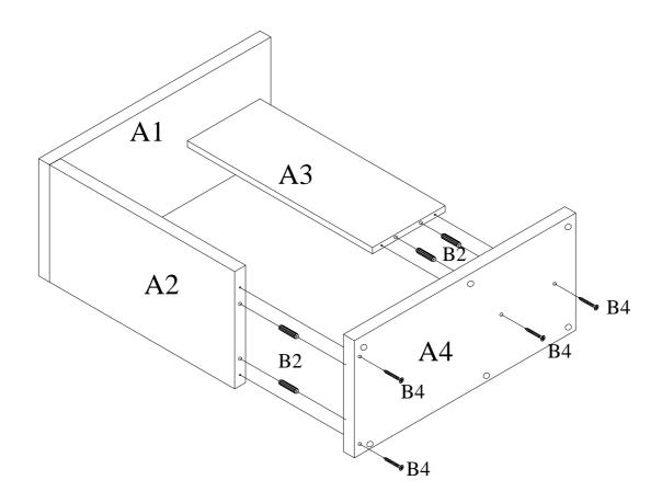
Assemble Bottom Panel A4 to Side Panel A2 & Divider A3 using Wood Dowels B2 & Screws B4 as shown above.
