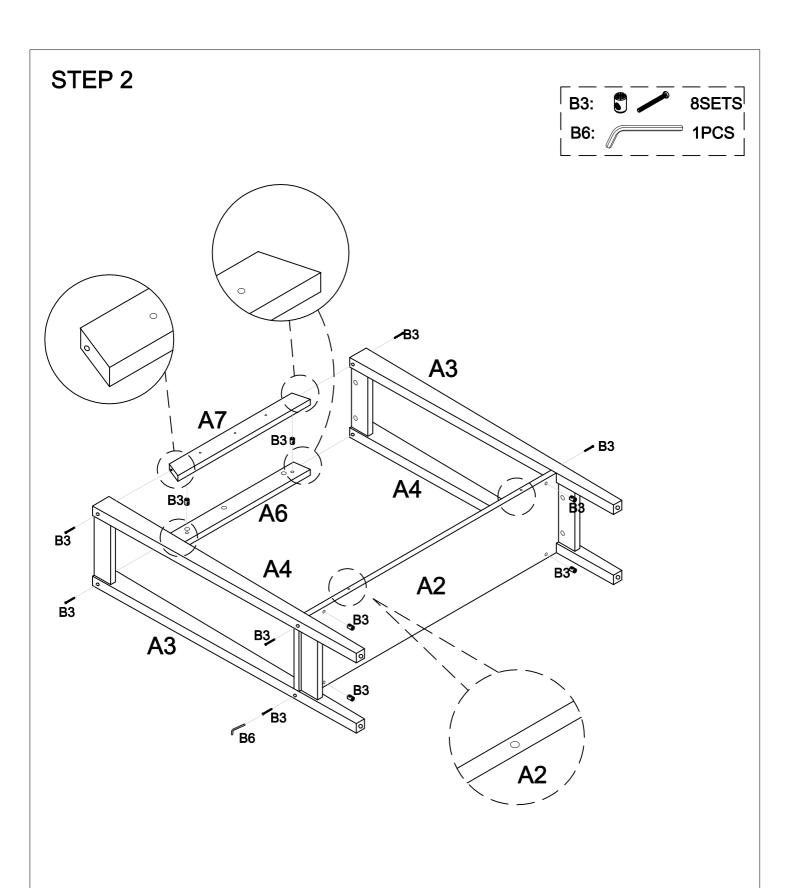
Assemble Aprons A6 &A7 and Shelf A2 to Legs A3&A4 using Bolts with nuts B3 as shown above.
