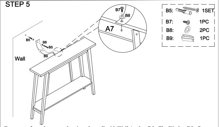
For your safety, please attach unit to the wall with Wall Anchor B5 , Flat Washer B8 , Screw B7 and Safety Wall Trap B9 as shown above.
