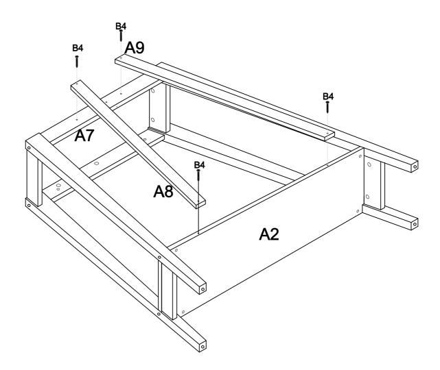
Assemble Support Bars A8 &A9 to Rear Apron A7 using Screws B4 as shown above.
