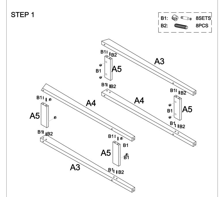
Assemble Connect Bars A5 to Legs A3 &A4 using Cam-locks B1 & Wood Dowels B2 as shown above.
