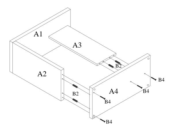
Assemble Bottom Panel A4 to Side Panel A2 & Divider A3 using Wood Dowels B2 & Screws B4 as shown above.
