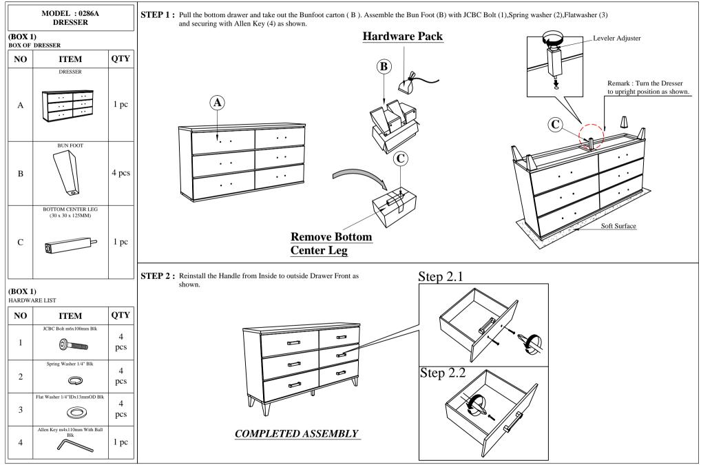
NOTE : MUST TIGHTEN SCREWS PERIODICALLY WITH USE SCREW WILL BECOME LOOSE CHECK TIGHTNESS OF ALL SCREW EVERY 6-8 WEEKS.
