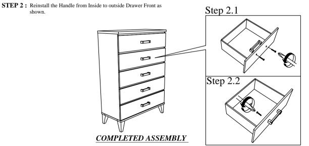
NOTE: MUST TIGHTEN SCREWS PERIODICALLY WITH USE SCREW WILL BECOME LOOSE CHECK TIGHTNESS OF ALL SCREW EVERY 6-8 WEEKS.
