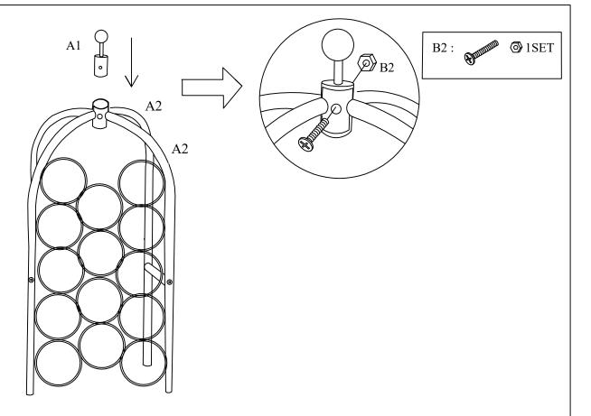
Insert Connect Block A1 into Side Frames A2 and tighten using Bolt with Nut B2 as shown above . Note: Please do not tighten bolt B2 until Step 3.
