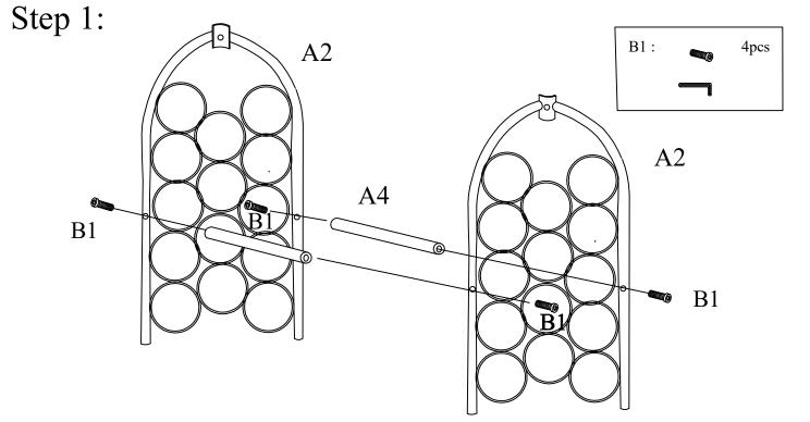
Assemble Side Frames A2 to Connect Bars A4 using Bolts B1 as shown above. Note: Please do not tighten bolts B1 until Step 3.
