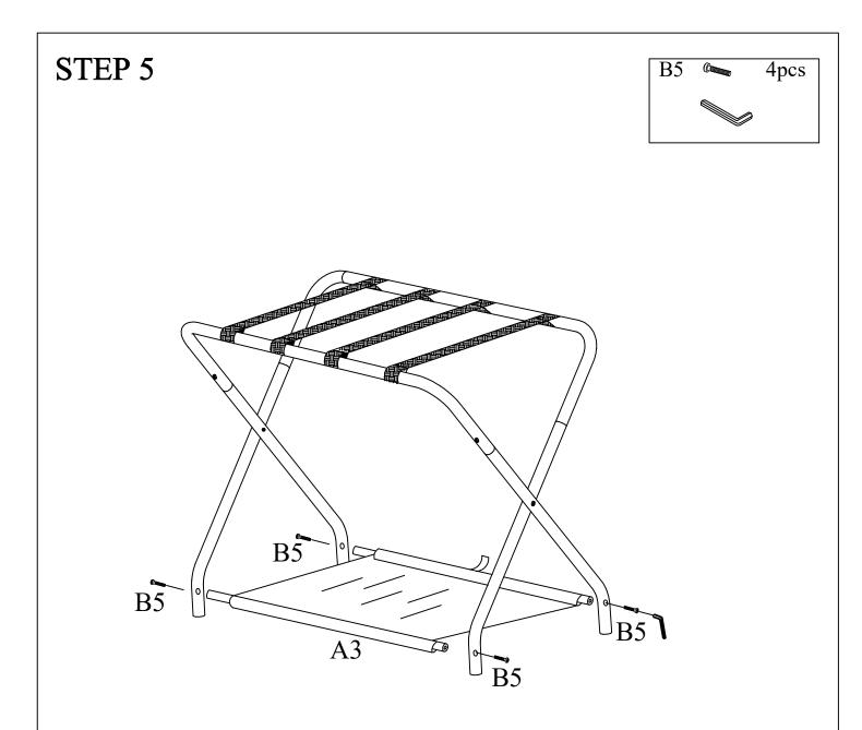
Assemble Shelf A3 to Legs A2 using Bolt B5 as shown above. Place the rack on the floor and check if it is stable before tightening bolts B1.
