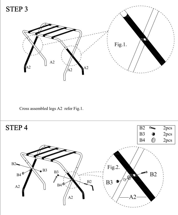
Assembled Legs A2 using Bolts B2, Washers B4 & Nuts B3 as shown above, please ensure washer B4 is inserted between legs A2, refer to Fig.2 (tighten bolts 90% at this point).
