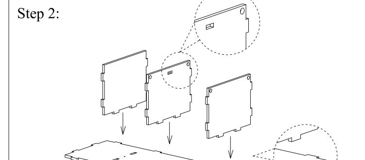
Attach the shelves to the back panel, by inserting them into the pre-drilled slats.
