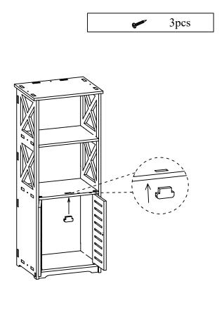
Insert the door stopper into holes on the center shelf as shown above.
