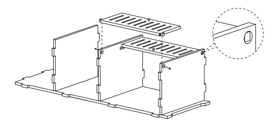
Attach the doors to the shelves, by inserting them into the pre-drillde slats as shown above.
