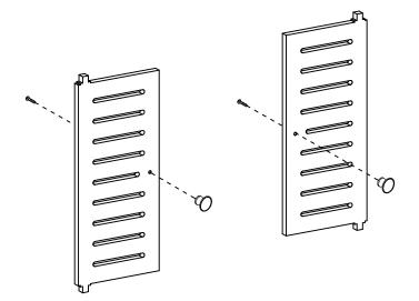
Attach the door knobs to doors using provided screws as shown above.
