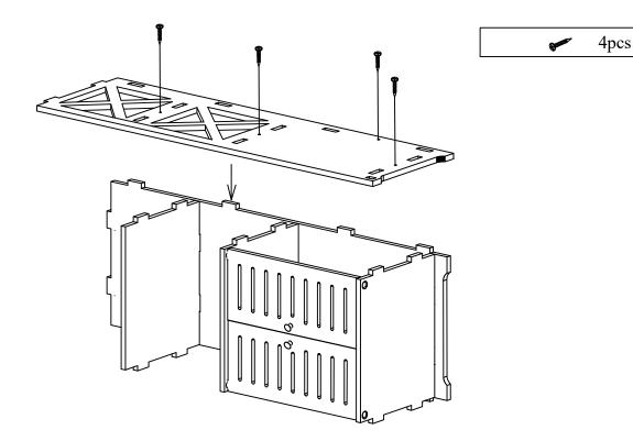
Attach the shelves and back panel to the side panel, by inserting them into the pre-drilled slats as shown above. Then tighten the side panel with provided screws into pre-drilled holes to secure unit as shown above.
