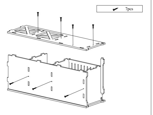
Attach the shelves and back panel to the other side panel, by inserting them into the pre-drilled slats as shown above. Then tighten the side panel & back panel with provided screws into pre-drilled holes to secure unit as shown above.
