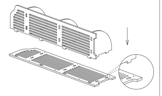
Attach the shelves and left side panel to the right side panel, by inserting them into the pre-drilled slats as shown above.
