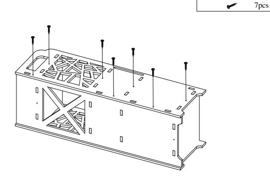
Insert and tighten left side panel with provided screws into pre-drilled holes to secure unit, as shown above.
