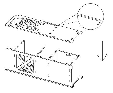
Attach the shelves to the left side panel, by inserting them into the pre-drilled slats as shown above.
