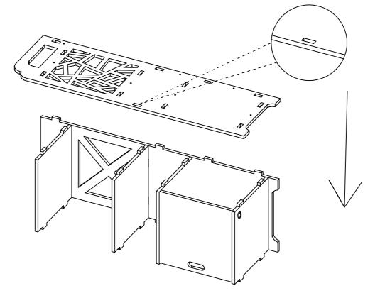
Attach the shelves to the right side panel, by inserting them into the pre-drilled slats as shown above.
