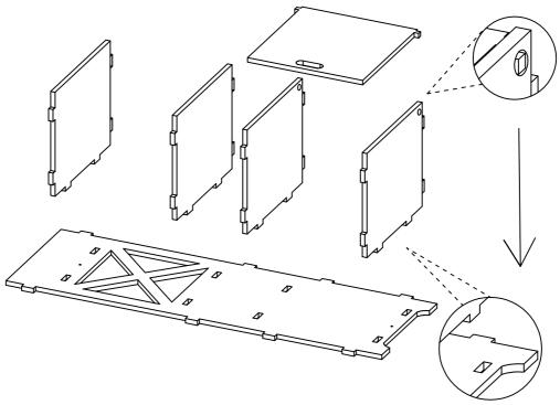
Attach the shelves to the back panel, by inserting them into the pre-drilled slats as shown above.
