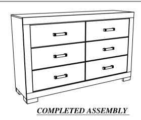
NOTE: MUST TIGHTEN SCREWS PERIODICALLY WITH USE SCREW WILL BECOME LOOSE CHECK TIGHTNESS OF ALL SCREW EVERY 6-8 WEEKS.
