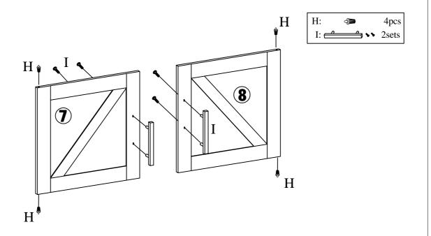
Insert Door Pins (H) into the hole on the two ends of Door Panels (7&8). Then attach Door Handles (I) to Door Panels (7&8) using included bolts (I).
