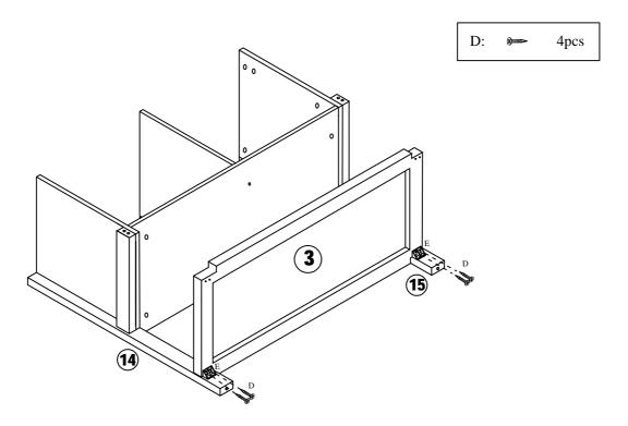
Assemble Bottom Shelf (3) to Rear Legs (14&15) using Screws (D) as shown above.
