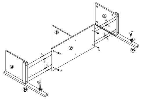
Assemble Divider Panel (2) to Side Panels (4&6) using Cam-Locks (A) and Wood Dowels (B) as shown above. Assemble Connect Block (E) to Rear Legs (14&15**)** using Screws (D) as shown above.
