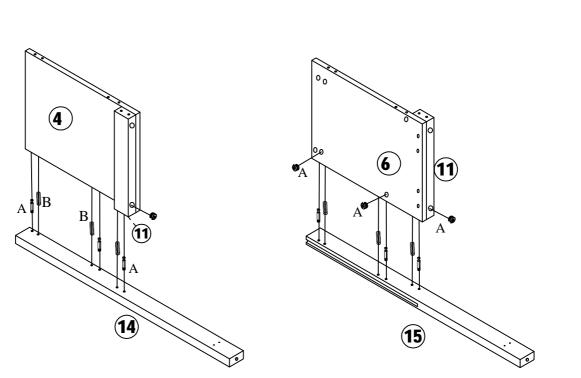
Assemble Rear Legs (14&15**)** to Side Panels (4&6) and Connect Bars (11) using Cam-Locks (A) and Wood Dowels (B) as shown above.
