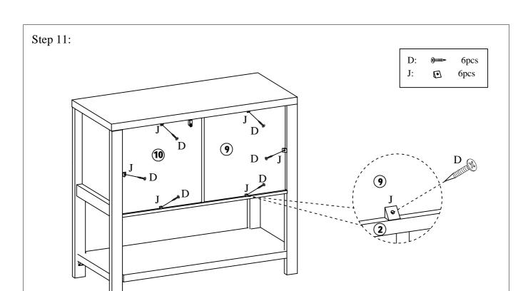
Attach Connect Blocks (J) to Rear Legs (14 &15) ,Divider (2) and Top Panel (1) to hold Back Panels (9&10) using Screws (D) as shown above.
