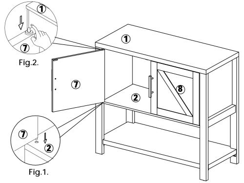
Connect Door Panels (7&8) to Divider Panel (2) as drawing Fig.1. Then press down Door Pin (H) ( see Fig.2.) and hold the Door Panel carefully into the cabinet with the upper pin popping up into the hole of Top Panel (1).
