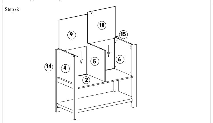
Insert Back Panels (9&10) into the grooves on Dividers (2&5), Rear Legs (14&15) as shown above.
