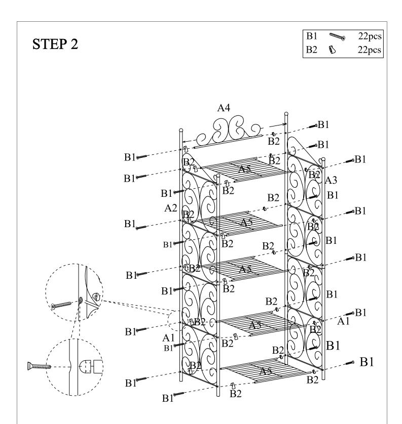
Assemble Net Rack A5 & Top Frame A4 to Side Frames A1&A2&A3 using Bolts B1 and Plastic Block B2 as shown above.
