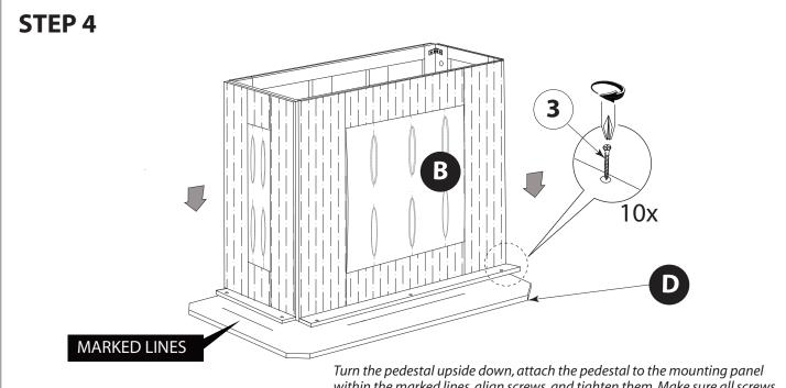
Turn the pedestal upside down, attach the pedestal to the mounting panel within the marked lines, align screws, and tighten them. Make sure all screws and connecting bolts are fully tightened before turning the table base upright, by two adults or more.
