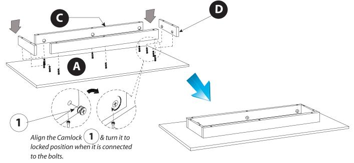
**STEP 3** Assemble the Legs to the Lower Panel B
