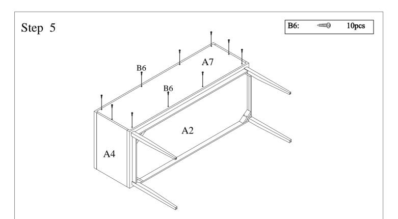
Assemble Back Panel A7 to the back of Side Panels A3 & A4, Top Panel A1 and Divider A5 using Screws B6 as shown above.
