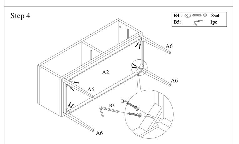
Assemble Legs A6 to Bottom Panel A2 using Bolts B4 with washers as shown above.
