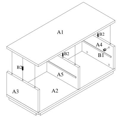
Assemble Top Panel A1 to Side Panels A3 & A4, Divider A5 using Cam-lock B1 and Wood Dowel B2 as shown above
