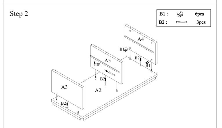
Assemble Side Panels A3 & A4 and Divider A5 to Bottom Panel A2 by Wood Dowel B2 and Cam-nut B1 with inserted Cam-bolts as shown above.
