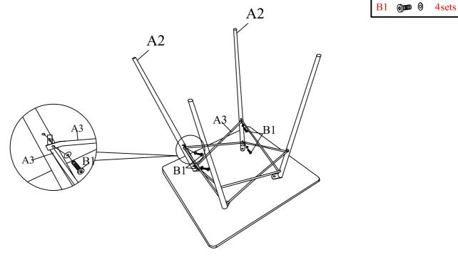
Assemble the other Connect Bars A3 to Legs A2 using Bolt with Washers B1 as shown above. Noted:Place the table on the floor and check if it is stable before tightening all bolts.
