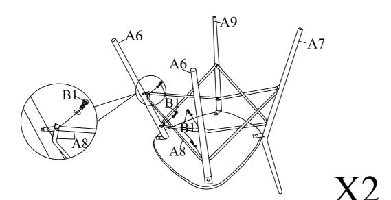
Assemble the other Connect Bars A8 to Front Legs A6 using Bolt with Washers B1 as shown above. Noted:Please do not tighten Bolts B1 until Step 7.
