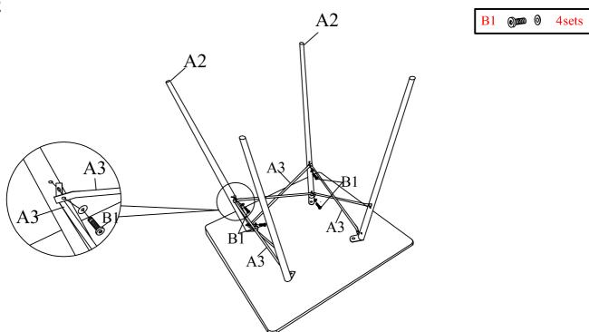
Assemble 3 pieces Connect Bars A3 to Legs A2 using Bolt with Washers B1 as shown above. Noted:Please do not tighten Bolts B1 until Step 3.
