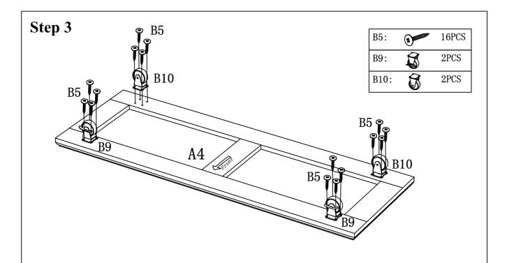
Assemble Caster with Brake B9 & Caster B10 to the bottom of Bottom Panel A4 using Screws B5 as shown above.
