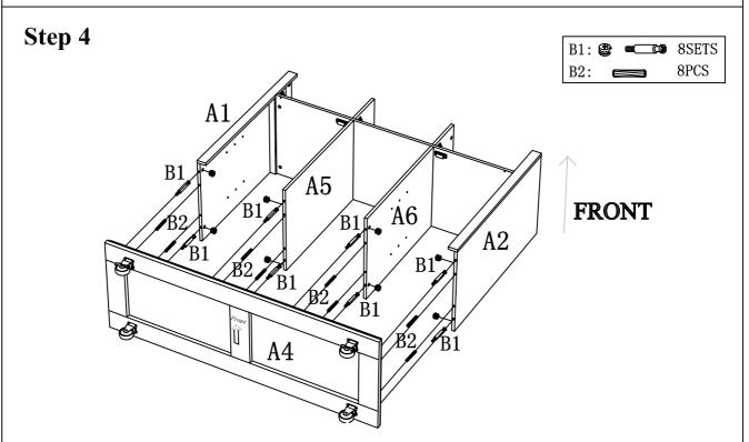
Assemble Bottom Panel A4 to Side Panels A1 &A1, Dividers A5 & A6 using Camlocks B1 and Wood Dowels B2 as shown above.
