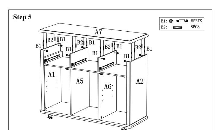
Assemble Top Panel A7 to Side Panels A1 &A2, Dividers A5 & A6 using Camlocks B1 and Wood Dowels B2 as shown above.
