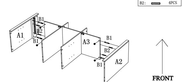
Assemble Side Panels A1 & A2 to Middle Shelf A3 using Camlocks B1 and Wood Dowels B2 as shown above.
