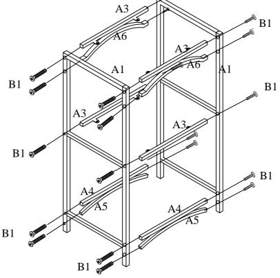
Attach Connect Bars (A3)&(A4) &(A5)&(A6) to Side Frames (A1) using Bolts (B1) as shown above. NOTE: Please do not tighten Bolts B1 until step 3.
