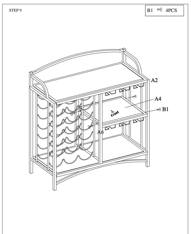
Assemble Shelf Frame A4 to Right Side Frame A2 and Divider A6 using Bolts (B1). Then tighten all bolts at this point.
