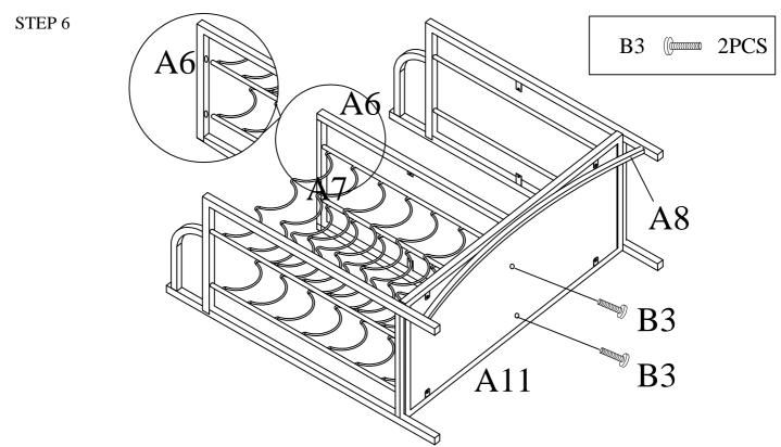
Insert Bottle Racks (A7) into holes on the top of Divider Frame (A6) .Then Attach Bottle Racks (A7) and Divider Frame (A6) to Bottom Panel (A11) using Bolts (B3). NOTE: Please do not tighten Bolts (B3) until step 9.
