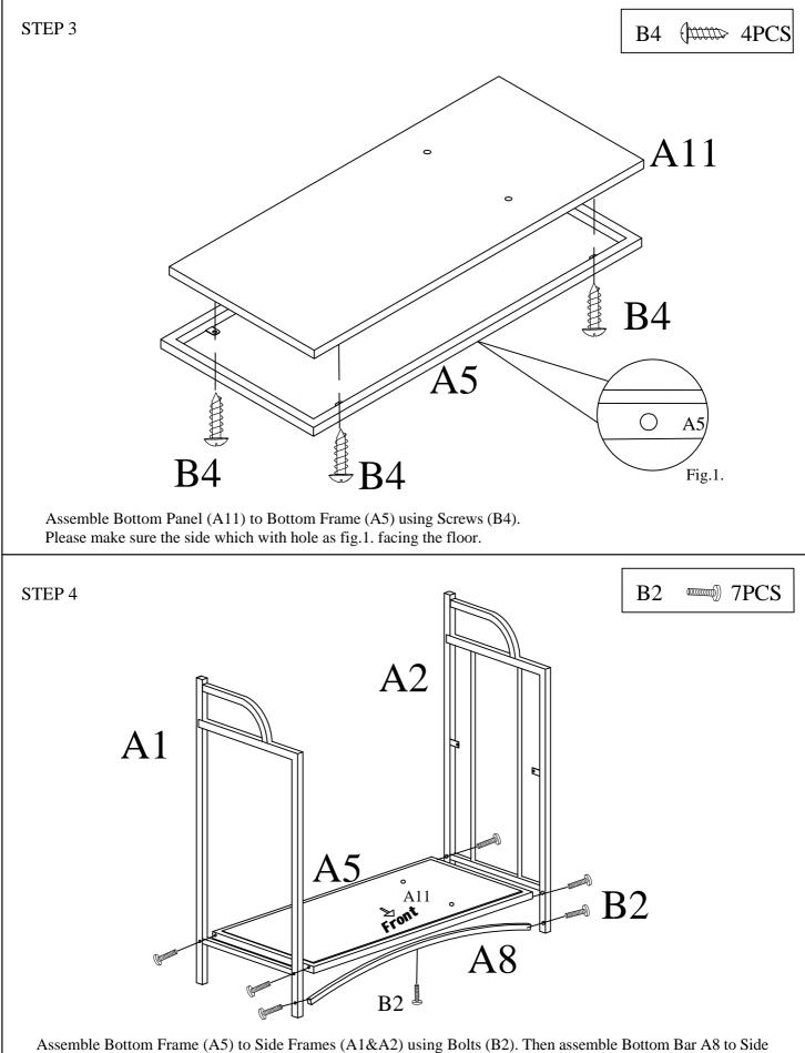
Assemble Bottom Frame (A5) to Side Frames (A1&A2) using Bolts (B2). Then assemble Bottom Bar A8 to Side Frames(A1&A2) and Bottom Frame (A5) using Bolts(B2). NOTE: Please do not tighten Bolts (B2) until step 9.
