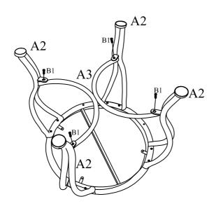
Attach Connect Frame A3 to Legs A2 using Bolts B1. Note: Please do not tighten Bolts B1 until Step 4.
