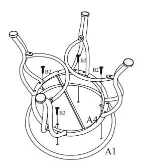
Assemble Seat Cushion A1 to Seat Frame A4 using Screws B2. Note:Please do not tighten Screws B2 until step 4.
