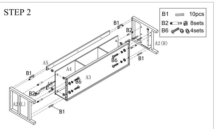
Assemble Side Frames A2(L&R) to Bottom Panel A3 ,Shelf Panel A4 and Upper Aprons A5 using Wood Dowels B1, Camlocks B2 and Bolts B6 with washers.
