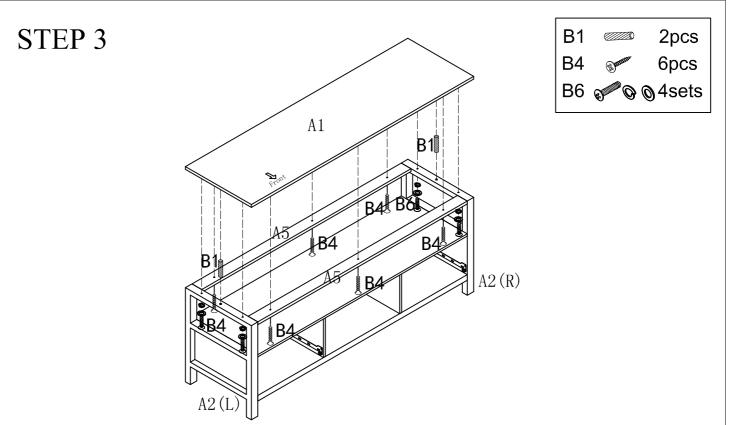
Assemble Top Panel A1 to Side Frames A2(L&R) ,Upper Aprons A5 using Wood Dowels B1,Screws B4 and Bolts B6 with washers.
