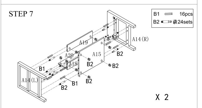
Assemble Side Frames A14(L&R) to Bottom Panel A15 ,Connect Bars A18 &A19, Back Panel A20 using Wood Dowels B1, Camlocks B2 as shown above.
