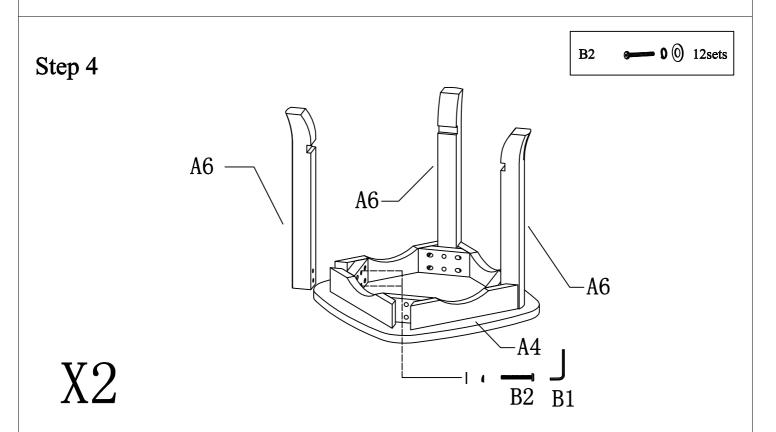
Assemble three Legs A6 to Top Panel A4 using Bolts with Washers B2. Please do not tighten Bolts B2 until step 6.
