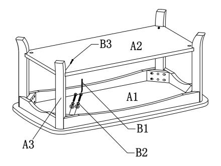
Assemble the 4th Leg A3 to Top Panel A1 using Bolts with Washers B2, then tighten Shelf A2 to the one Leg A3 using Screw B3. Place the table on the floor and check if it is stable before tightening all bolts.
