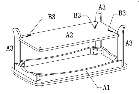
Insert Shelf A2 into the grooves on Legs A3, then tighten Shelf A2 to Legs A3 using Screws B3. NOTE: It is recommended that this step should be assembled by two persons.
