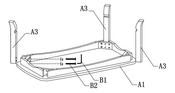
Assemble three Legs A3 to Top Panel A1 using Bolts with Washers B2. Please do not tighten Bolts B2 until step 3.
