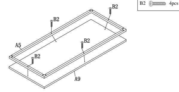
Assemble Top Panel A9 to Top Frame A5 using Bolts B2.
