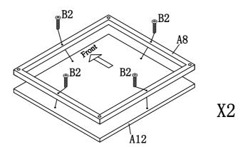
Assemble Shelf A12 to Shelf Frame A8 using Bolts B2.
