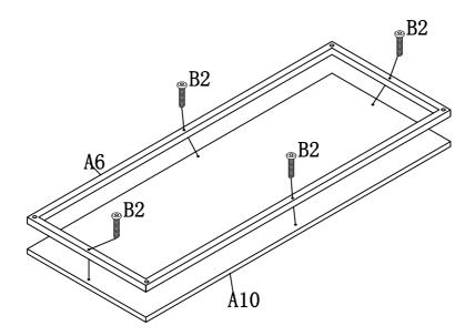
Assemble Shelf Panel A10 to Shelf Frame A6 using Bolts B2 .
