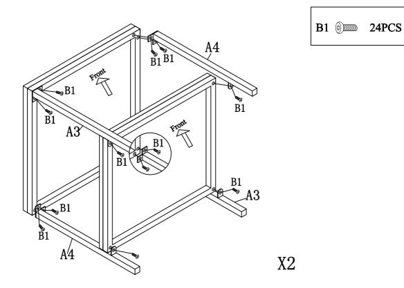
Assemble Legs A3&4to Top Frame A7 using Bolts B1 . Then assemble Shelf Frame A8 to Legs A3&4 using Bolts B1 .
