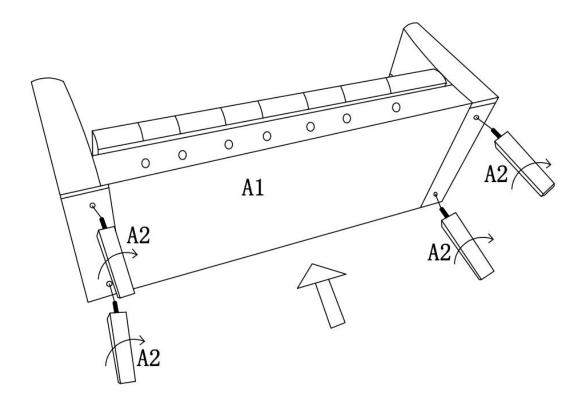
Attach Legs A2 to the bottom of Top Seat A1 as shown above.
