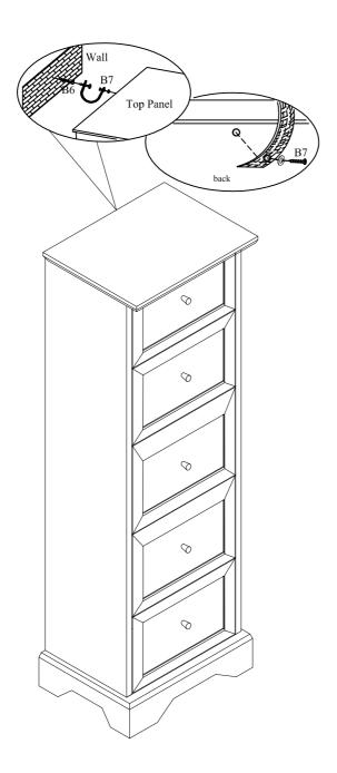
For your safety, please attach this unit to the wall by Anchor with screw B6 and Anti-tip Kit B7.
