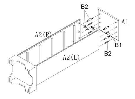
Attach Top Panel A1 to Side Panels A2(L&R) using Wood Dowels B1 and Cam-Locks B2.
