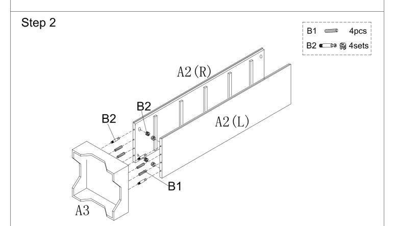
Assemble Side Panels A2(L&R) to Bottom Frame A3 using Wood Dowels B1 and Cam-Locks B2.
