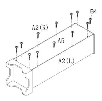
Attach Back Panel A5 to the back of the unit using Screws B4.
