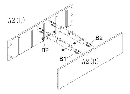
Assemble Side Panels A2(L&R) to Dividers A4 using Wood Dowels B1 and Cam-Locks B2.
