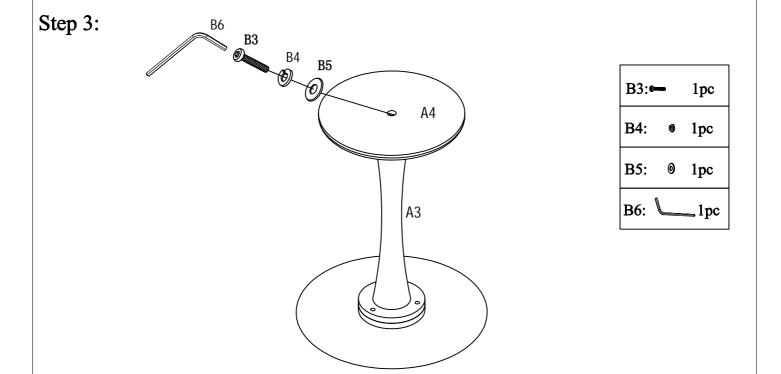
Assemble the base A4 to support bar A3 using bolt B3 with spring washer B4& flat washer B5.
