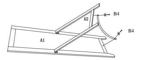
$Step \ 3: \ Attach \ Connect \ Bat \ A2 \ and \ the \ bottom \ of \ Mirror \ Frame \ A1 \ using \ included \ screws.$
