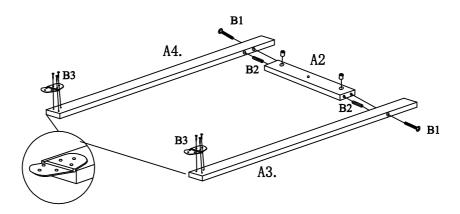
Step 1: Assemble Connect Bar A2 to Legs A3 & A4 using Bolt with nuts B2 and Wood Dowels B2 as shown above.
