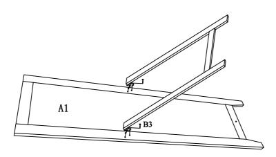
Step 3: Assemble Hinges B3 to Mirror Frame A1 using included screws as shown above.
