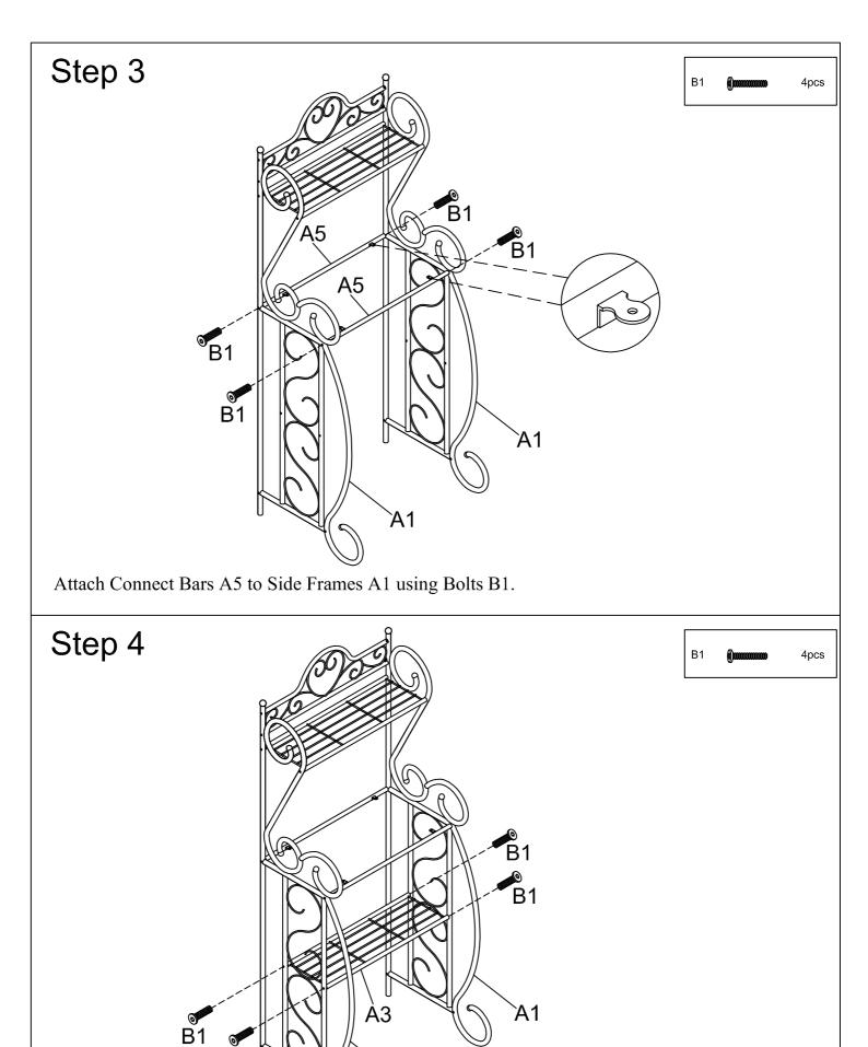
Attach Upper Rack A3 to Side Frames A1 using Bolts B1.
