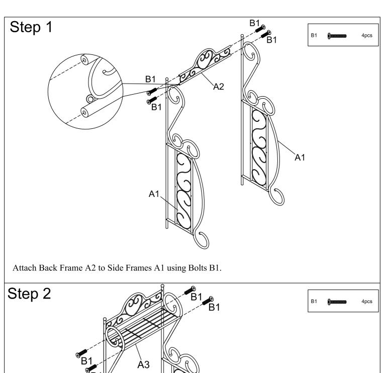
Attach Upper Rack A3 to Side Frames A1 using Bolts B1.
