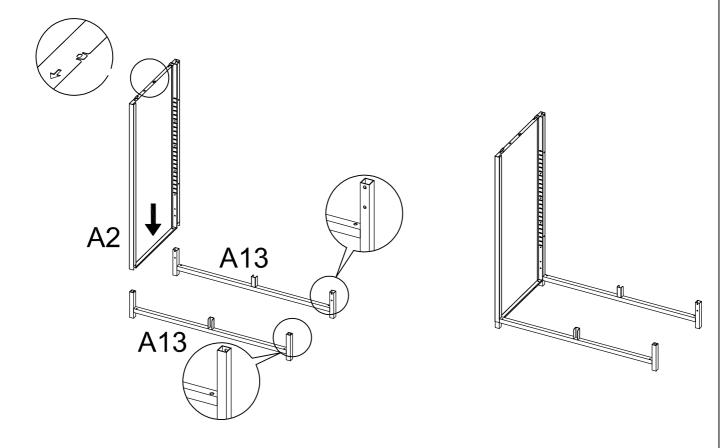
Insert Left Side Panel A2 into Connect Frames A13 as shown above.
