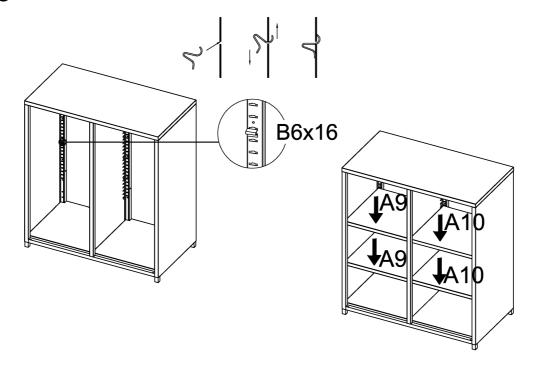
Attach Hooks B6 to Side Panels A2&A3 and Divider A6 as shown above, then place Shelf Panels A9&A10 into the unit.
