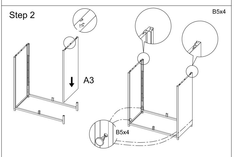
Insert Right Side Panel A3 into Connect Frames A13, then tighten them using Caps B5 as shown above.
