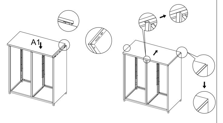
Attach Top Panel A1 to Side Panels A2&A3 (L&R), Back Panels A4&A5 (L&R) and Divider A6 as shown above.
