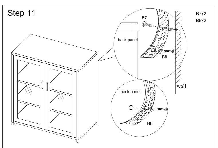
For your safety, please attach the unit to the wall by Anchors with screws B7 and Anti-tip kits B8.
