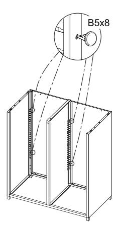
Assemble Back Panels A4&A5 (L&R) to Side Panels A2&A3 (L&R), Divider A6 and Connect Frame A13, then tighten them using Caps B5 as shown above.
