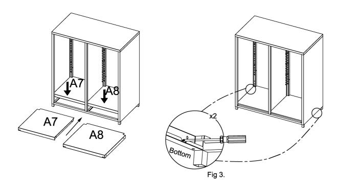
Insert Bottom Panels A7 & A8 (L&R) into the unit, then place the unit down on the floor carefully and tighten Bottom Panels A7&A8 (L&R) to Side Panels A2&A3 (L&R) by folding the metal plates, refer to Fig 3.
