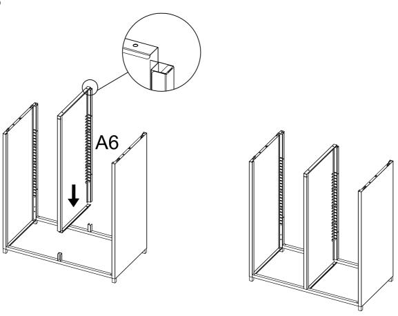
Insert Divider A6 into Connect Frames A13 as shown above.
